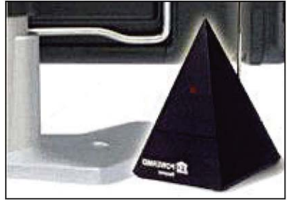
Figure 26. A RF TV remote can cause interference
