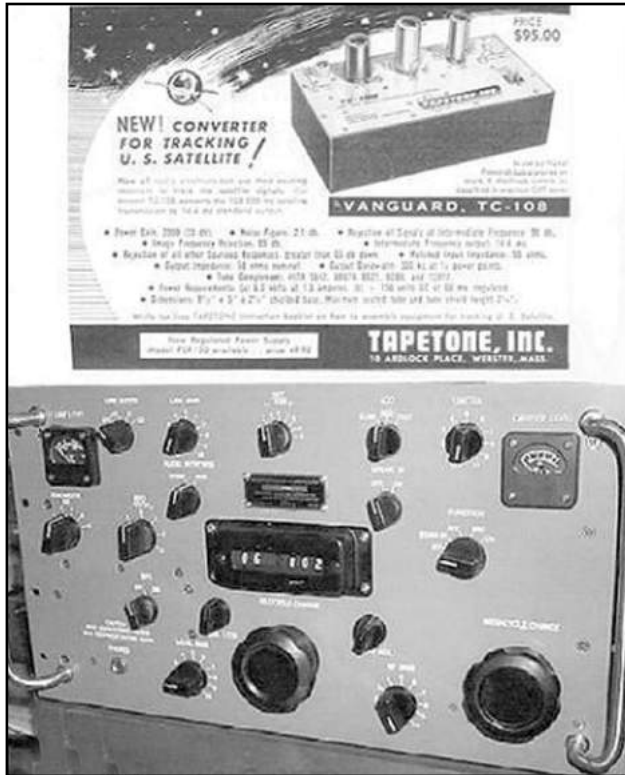
Photo 28-2.20. TIROS 1 108-MHz Telemetry Data Receiver at RCA's Ground Station at Princeton, New Jersey.
