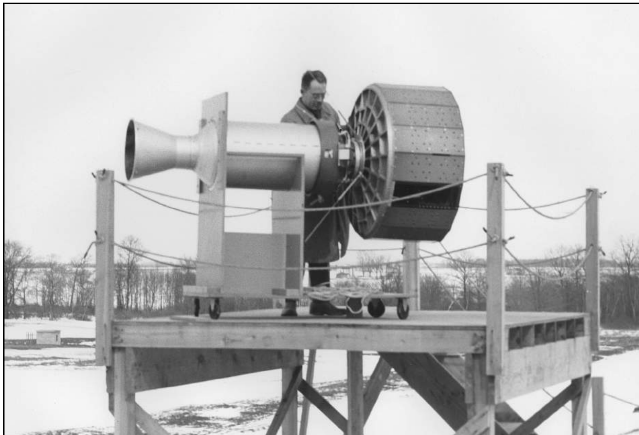
Photo 28-2.8. The author assembling an electrical test model of TIROS 1 to an empty third-stage booster rocket in 1959 in preparation for taking antenna radiation patterns to determine the effect of the rocket on the radiation patterns of the spacecraft antenna system.
