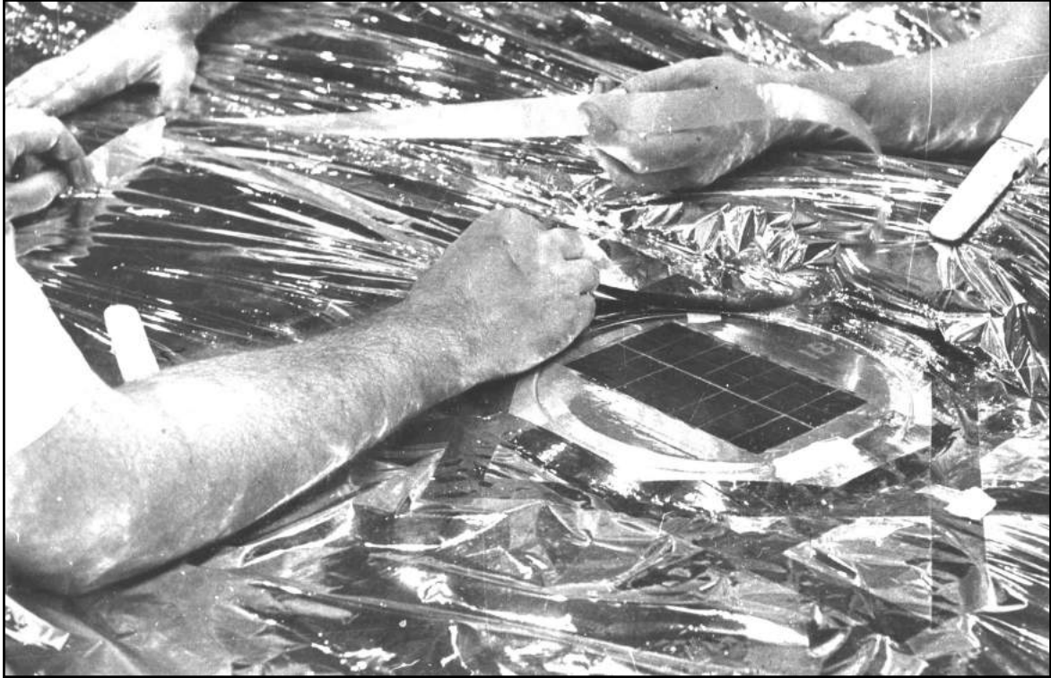
Photo 28-3.4. Beacon unit being attached to Echo 1 balloon satellite (aluminum-coated mylar) prior to balloon being folded in preparation for launch configuration.
