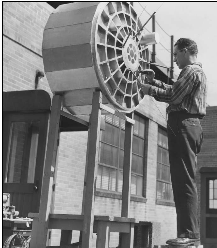
Photo 28-2.7. This picture, taken in 1959 at the Antenna Lab of the RCA Laboratories (David Sarnoff Research Center), shows the full-scale TIROS 1 electrical-test model, with author Maxwell working on the four-monopole transmitting antenna array during its development.
