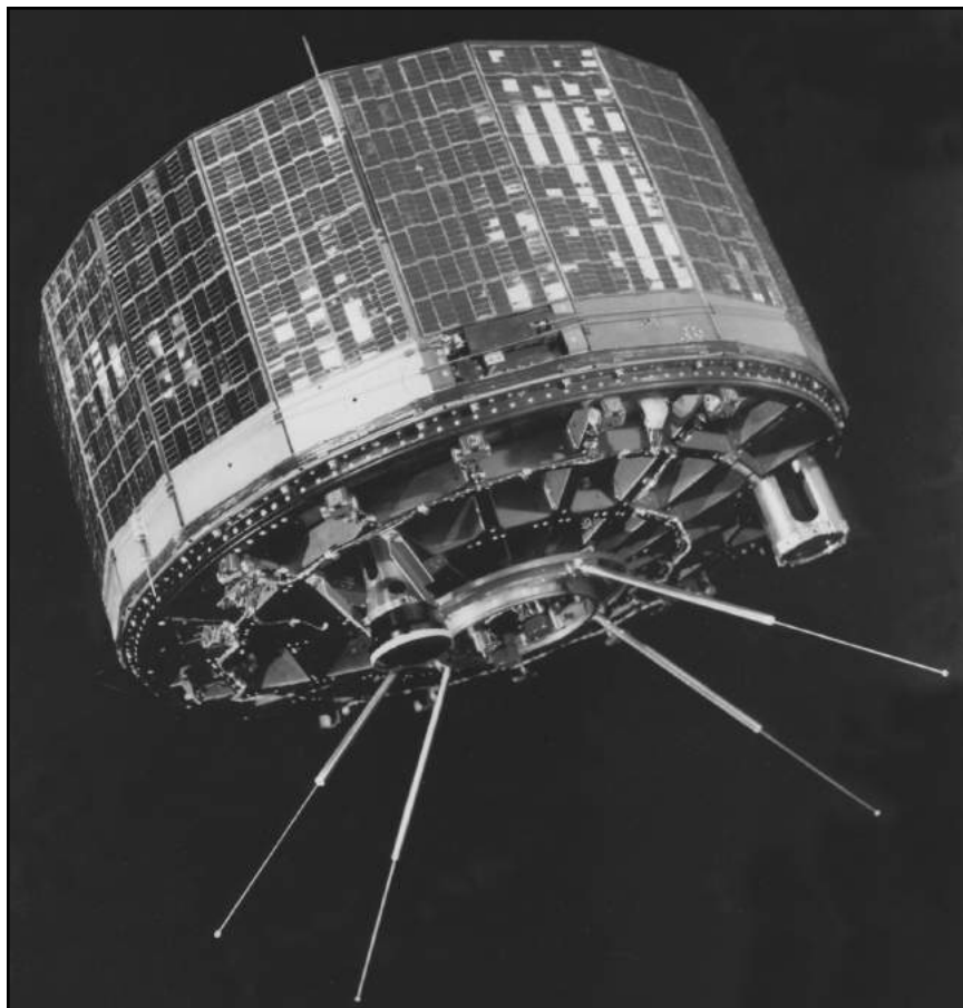
Photo 28-2.1. TIROS 1 weather satellite showing solar cells, cameras, and the author's multi-frequency transmitting antenna array.
