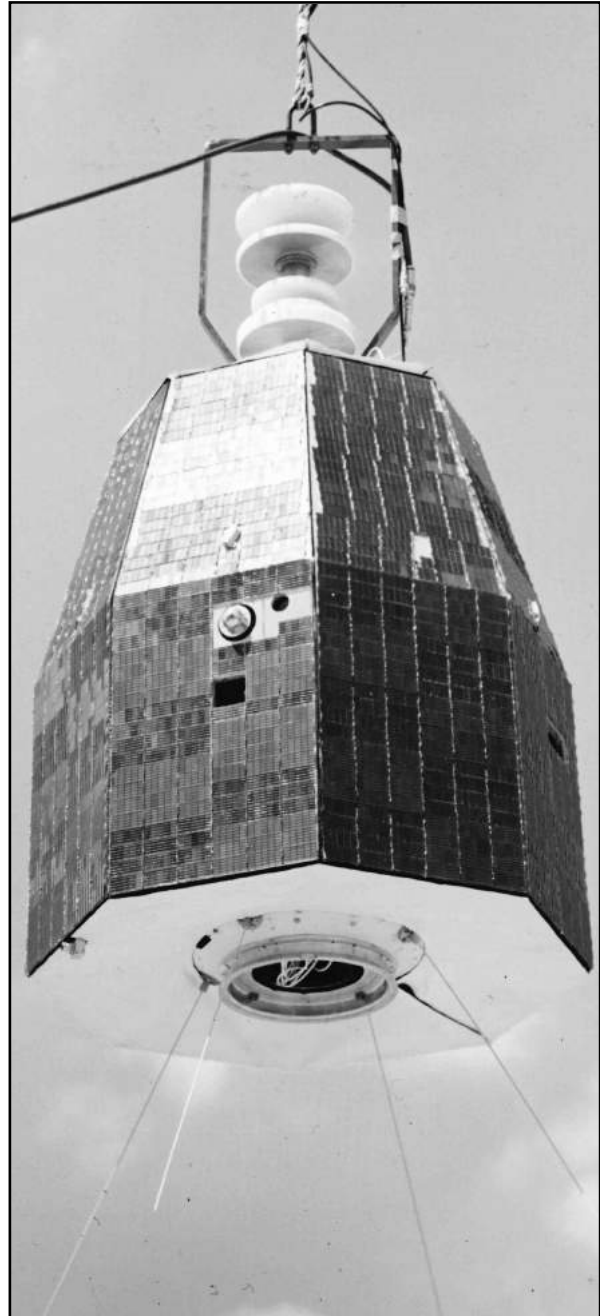
Photo 28-4.1. The RELAY Communications Spacecraft. The white disks at the top of the spacecraft are data-transmission (TV) antennas. The top disk is the 1.726-GHz receiving antenna, right-hand circular polarization (RHCP). The lower disk is the 4.71-GHz transmitting antenna, left-hand circular polarization (LHCP). The four monopoles at the bottom of the spacecraft are the antennas for receiving commands from the ground stations on 148 MHz, and transmitting telemetry data to the ground stations on 136 MHz.
