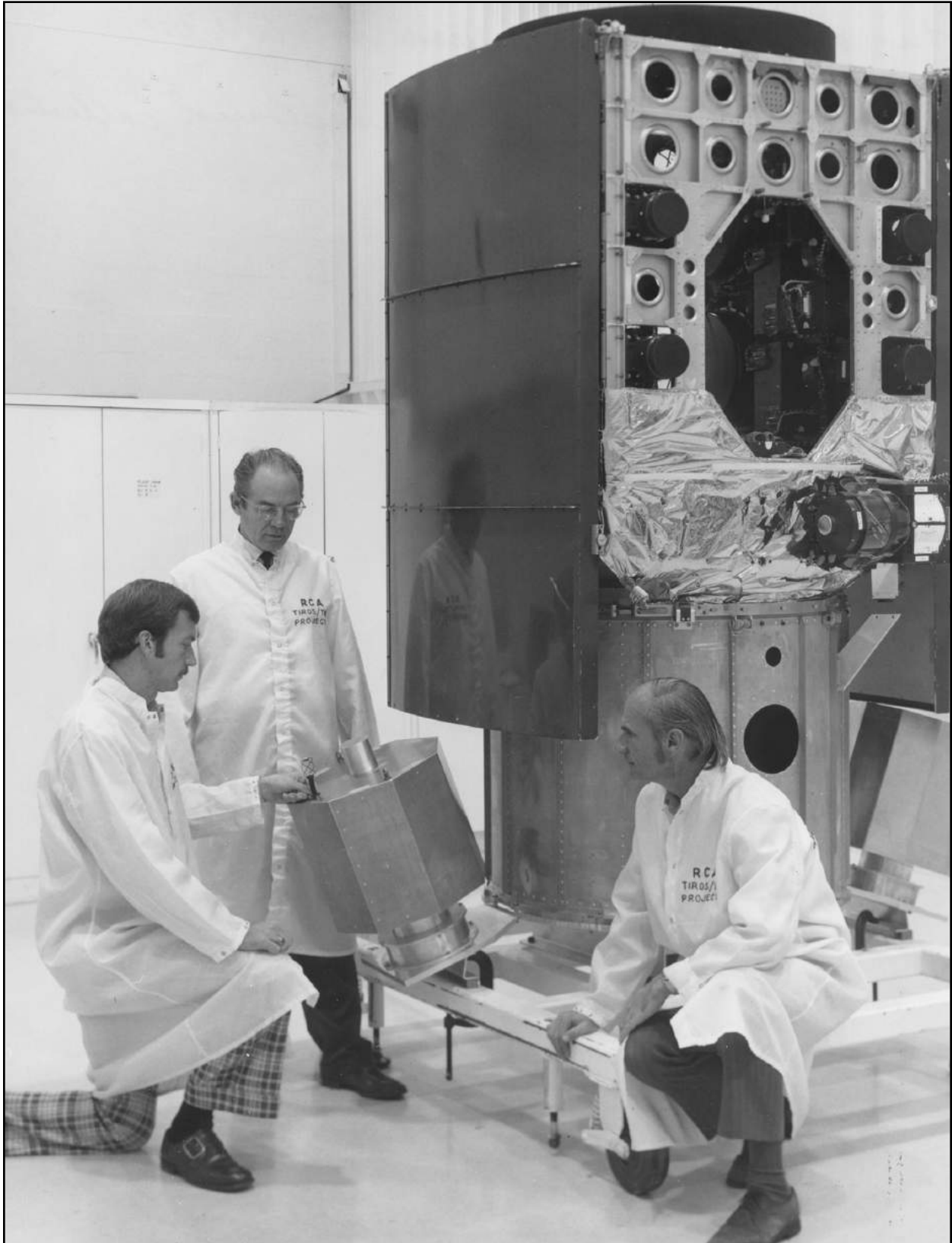
Fig 22-13. OSCAR 7 test model with TIROS 9 spacecraft while under construction at RCA Space Center, Princeton (Hightstown), New Jersey.
