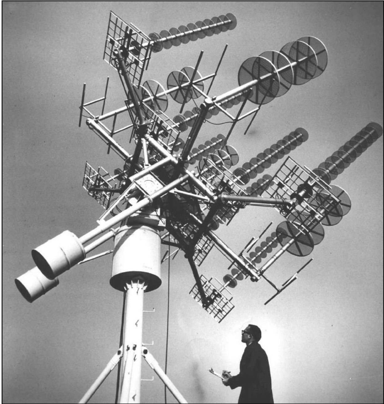
Photo 28-2.18. Az-El high-gain TIROS tracking Antenna at RCA's ground station at Princeton, New Jersey.
