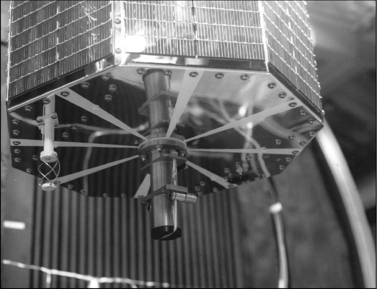
Fig 22-16. Bottom view of OSCAR 7 showing close-up view of the RCA-donated quadrifilar helix beacon antenna designed by the author.
