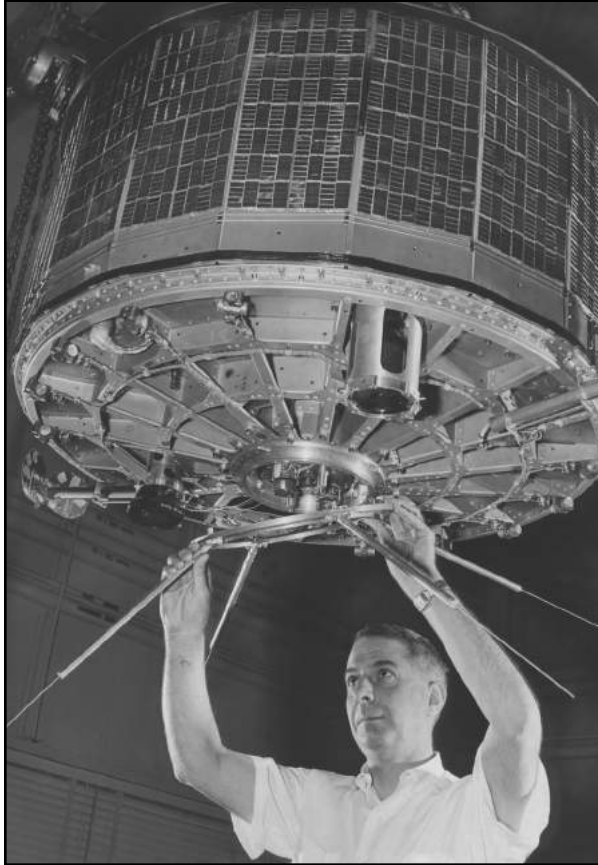
Photo 28-2.9. RCA mechanical technician Herb DeCerro attaching the author's antennas to the TIROS 1 spacecraft.
