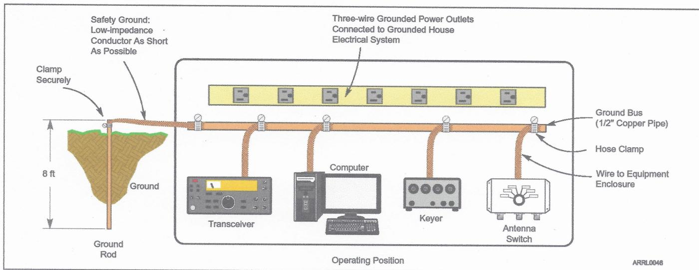
**Figure 2** — The ground bus shown in this figure provides effective bonding between the various pieces of equipment at RF. The ac safety ground is also connected to the ground bus, but is of limited effectiveness at RF.
