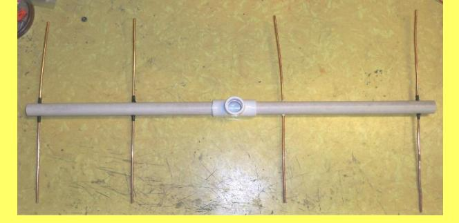
Drill the PVC boom and insert the elements. Note the 'TEE' in the middle for mounting the antenna.
