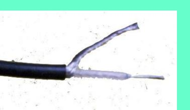
Twist and tin the braid. Cut 3/8" Off the center insulation and tin The center conductor.
