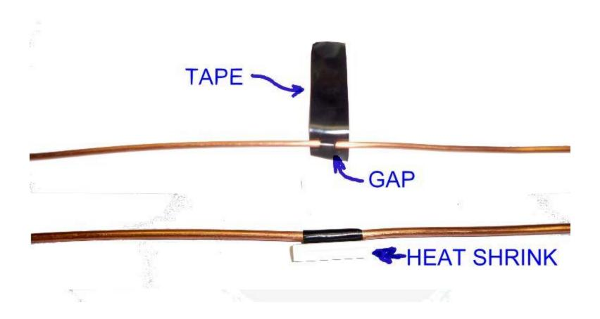
Prepare the driven element leaving a ¼" gap. Tape it and secure it with heat shrink. You may have to re-cut the element to length.
