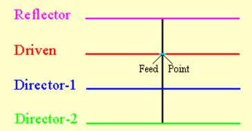
4 element yagi easy to build and feed directly with 50 ohm coax.
