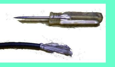
With a pointed tool, comb out the Braid away from the cener conductor.
