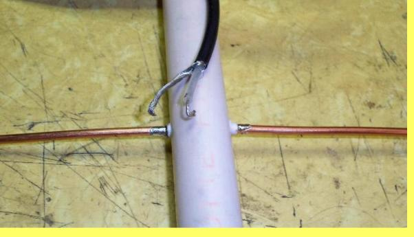
Bend the tinned wires to fit over the driven element... Tin the driven element where you will attach the coax. DO NOT USE EXCESSIVE HEAT!
