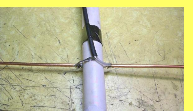
Solder the coax to the driven element and tape the coax to the boom in two places.
