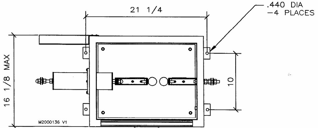
**Figure C-3 NAX185 Enclosed High Voltage Spark Gap**
