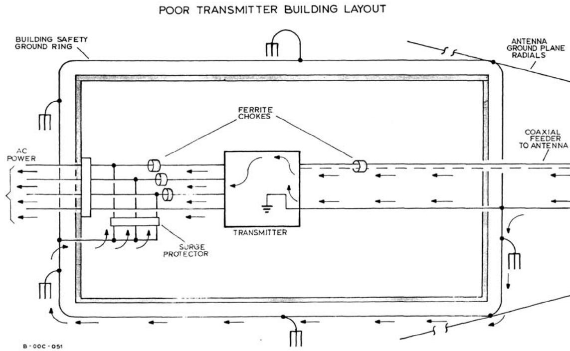
**Figure 6 Poor Transmitter Building Layout**
