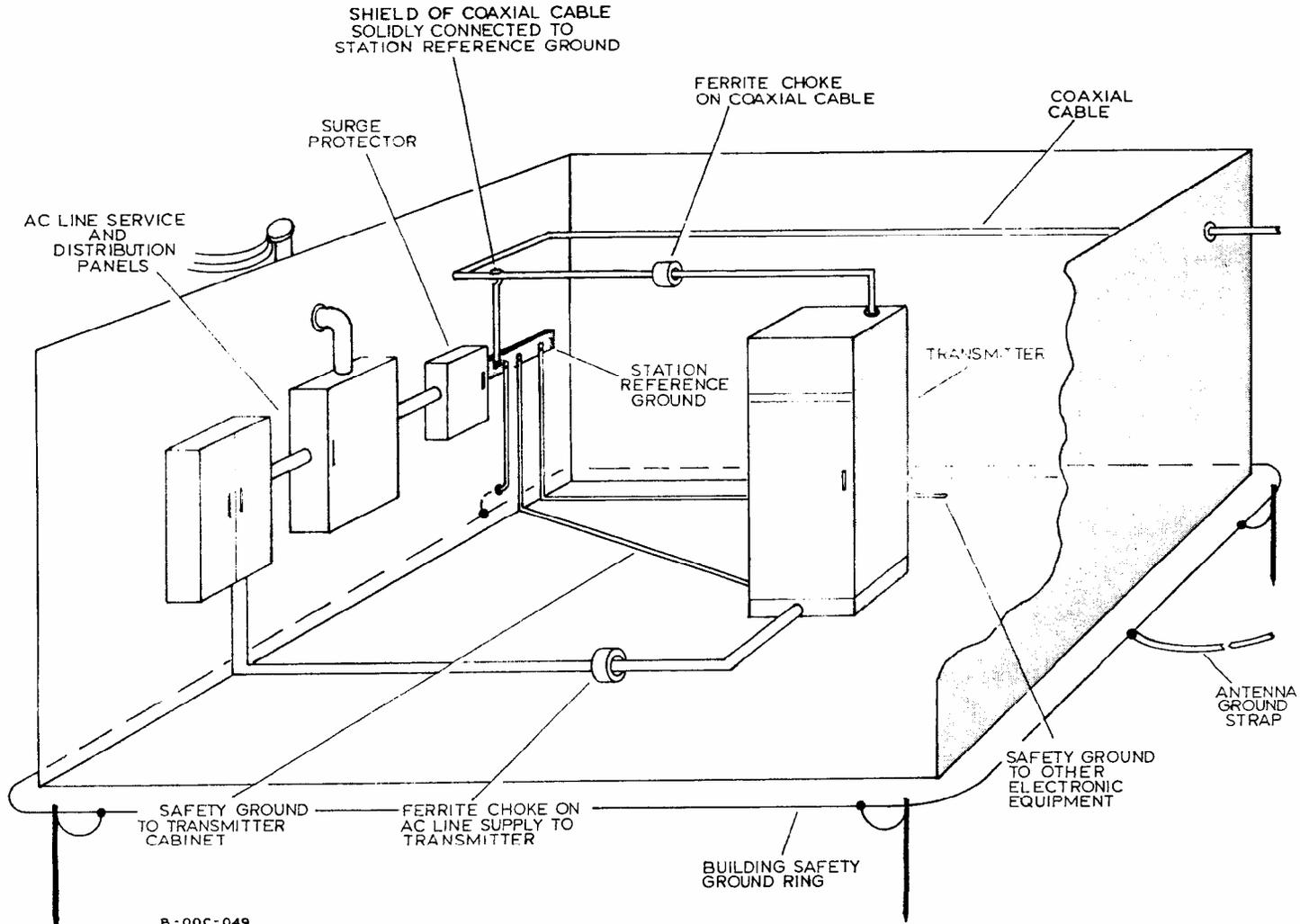
**Figure 7 Correcting A Poor Transmitter Building Layout**
