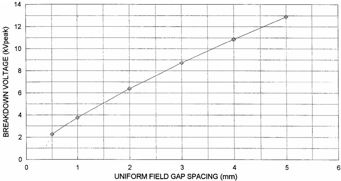
**Figure B-4 Determination of Uniform Field Gap Spacing (Low Volts - Less Than 14 kV<sub>PEAK</sub>)**
