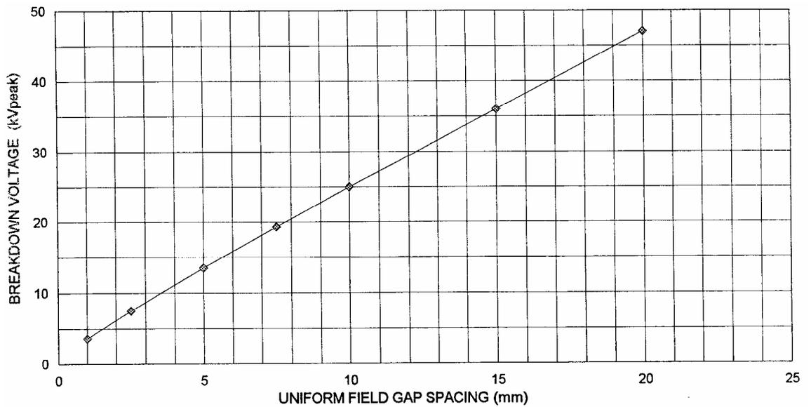
**Figure B-3 Determination of Uniform Field Gap Spacing (High Volts - Up to 50 kV<sub>PEAK</sub>)**
